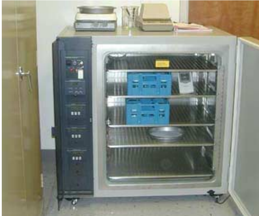
Figure 002: Interior of the incubator showing side panel controls, internal RH and Temperature monitor, and samples.
