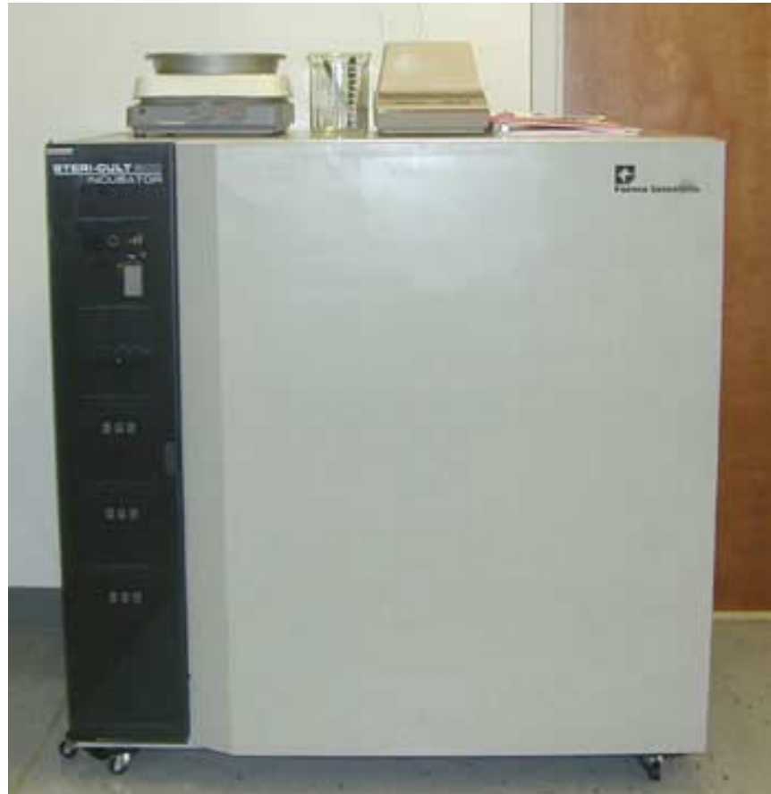
Figure 001: Forma Stericult 200 Model 3033 HEPA Filtered CO2/RH/Temp Incubator to control temperature and relative humidity for Water Vapor Transmission Rate Tests (WVTR).
