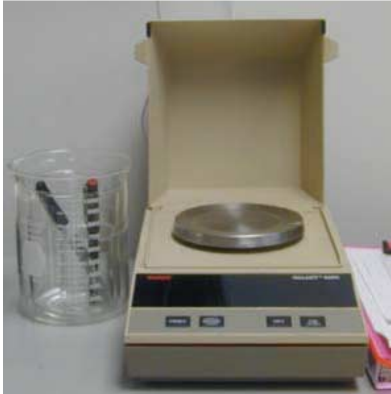
Figure 005: Ohaus Galaxy 400D Balance (Accuracy .001) Model G400DO to monitor the amount of water lost by evaporation through the stone.
