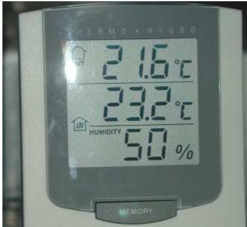
Figure 003: Internal RH and Temperature monitor. Test was run with an average 50% \pm 5% RH and a constant 23.3°C \pm 0.5°C.
