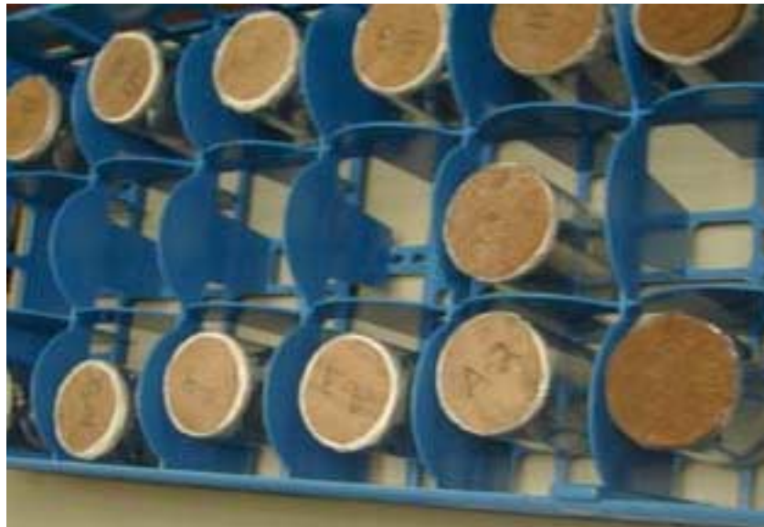
Figure 004: The edges of the sandstone sample disks were sealed with Teflon plumber's tape and then mounted in the top of a polypropylene vial filled with distilled water to a level \frac{3}{4} inch below the sample. The gap between the edge of the beaker and the sample was then sealed with Ethylene Vinyl Acetate.
